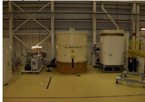
Helium Leak Test Vacuum Chamber (Step 19)
