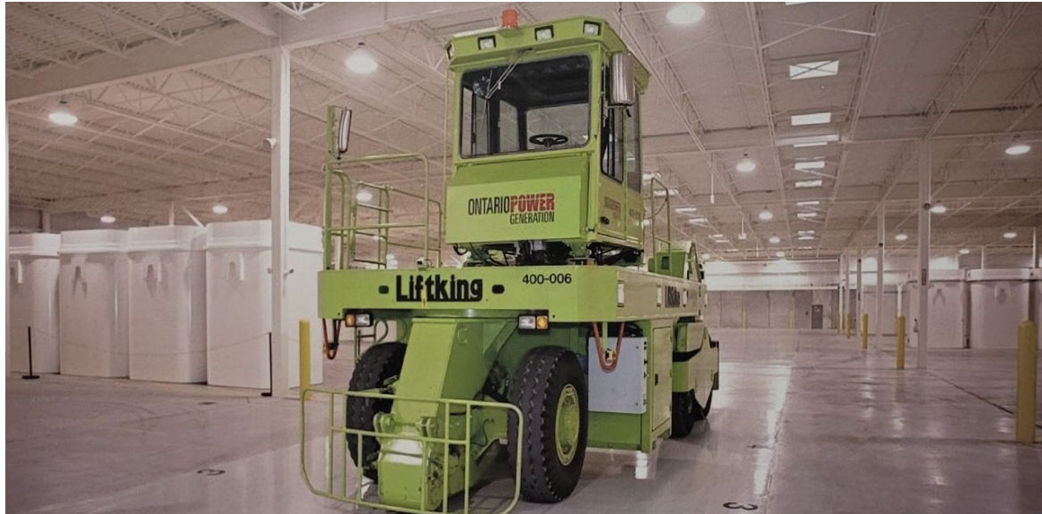
Figure 8: DSC Transporter in the NSS-D Used Fuel Dry Storage Building
